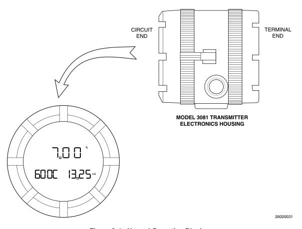
Figure 3-4. Normal Operation Display
